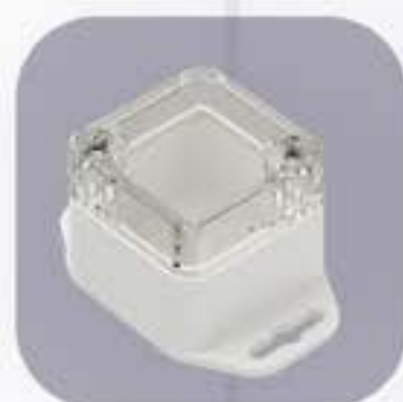
ZP45.45.40SU MATERIAL: ABS/ PC WITH FOAM GASKET H / W / L (mm): 40 / 45 / 45 AVAILABLE COLOURS: ■ ■
