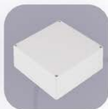
ZP150.150.60 MATERIAL: ABS/PC WITH GASKET H / W / L (mm): 60 / 149,9 / 149,9 AVAILABLE COLOURS: ■ ■
