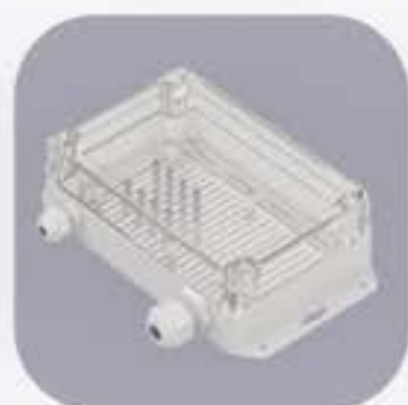
IOT.ZPSET1812.2 MATERIAL: PC WITH FOAM GASKET H / W / L (mm): 60,1 / 121,5 / 180,1 AVAILABLE COLOURS:
