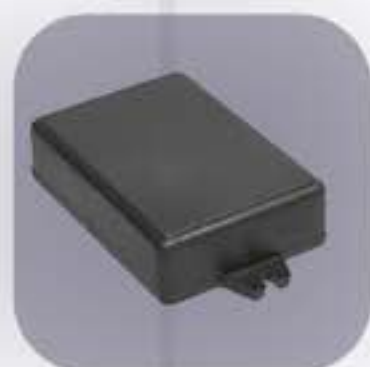
Z23U MATERIAL: PS/ABS H / W / L [mm]: 23,4 / 59,5 / 84,9 (106,7) FOR POWER SUPPLIES AVAILABLE COLOURS: ■
