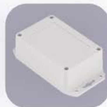
Z128SU MATERIAL: ABS WITH FOAM GASKET H / W / L [mm]: 40 / 70 / 105 AVAILABLE COLOURS: ■ ■
