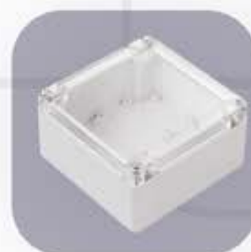
ZP120.120.60S MATERIAL: ABS/ PC WITH FOAM GASKET H / W / L (mm): 60,1 / 119,8 / 119,8 AVAILABLE COLOURS: ■ ■
