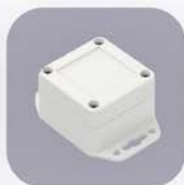
ZP60.60.40SU MATERIAL: ABS/ PC WITH FOAM GASKET H / W / L (mm): 40 / 60 / 60 AVAILABLE COLOURS: ■ ■
