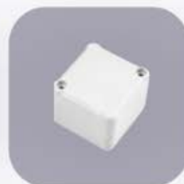
Z116 MATERIAL: PS/ ABS WITH GASKET H / W / L (mm): 36,2 / 48,9 / 51 AVAILABLE COLOURS: ■ ■
