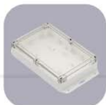
ZP210.140.45SU MATERIAL: ABS/ PC WITH FOAM GASKET H / W / L [mm]: 45 / 139,8 / 209,7 AVAILABLE COLOURS: ■ ■
