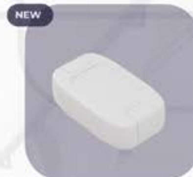
ZM110.70.33 MATERIAL: ABS FOR WALL MOUNTING H / W / L [mm]: 33 / 70 / 110 AVAILABLE COLOURS: [ ] [ ] [ ]
