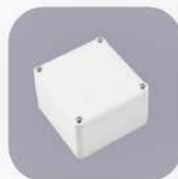
Z11S MATERIAL: ABS WITH FOAM GASKET H / W / L [mm]: 55 / 80 / 82 AVAILABLE COLOURS: ■ ■
