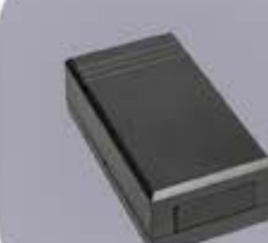
Z36 MATERIAL: PS/ABS H / W / L (mm): 42 / 66 / 125 WITH SIDE PANELS AVAILABLE COLOURS:
