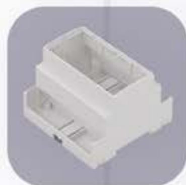
ZD1005 MATERIAL: ABS V0 H/ W / L (mm): 65 / 90 / 90 AVAILABLE COLOURS:
