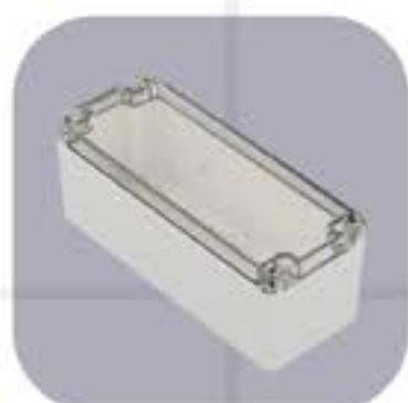
ZP190.75.75S MATERIAL: ABS/ PC WITH FOAM GASKET H / W / L [mm]: 75 / 75 / 190 AVAILABLE COLOURS: ■ ■
