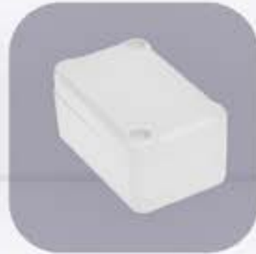
Z65 MATERIAL: PS/ ABS WITH GASKET H / W / L (mm): 30,1 / 40,1 / 64,4 AVAILABLE COLOURS: ■ ■
