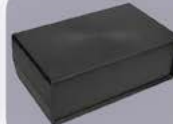
Z15 MATERIAL: ABS H / W / L (mm): 90 / 148 / 250 WITH SIDE PANELS AVAILABLE COLOURS:
