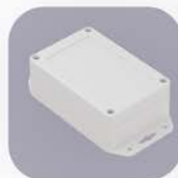
ZP120.80.45SU MATERIAL: ABS/ PC WITH FOAM GASKET H / W / L (mm): 45,2 / 81,6 / 121,4 AVAILABLE COLOURS: ■ ■
