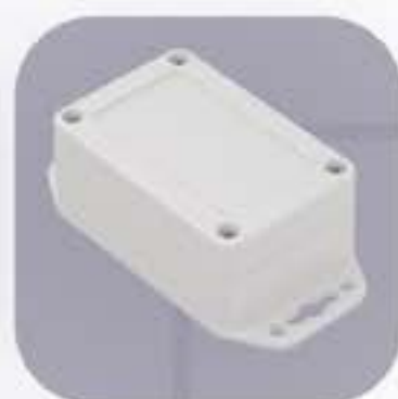
ZP90.60.40SU MATERIAL: ABS/ PC WITH FOAM GASKET H / W / L (mm): 39,9 / 61,3 / 90 AVAILABLE COLOURS: ■ ■
