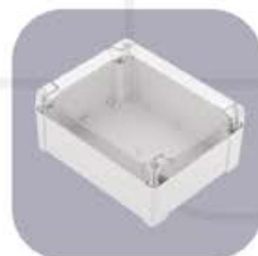
ZP240.190.105S MATERIAL: ABS/ PC WITH FOAM GASKET H / W / L [mm]: 105,7 / 191,3 / 240 AVAILABLE COLOURS: ■ ■
