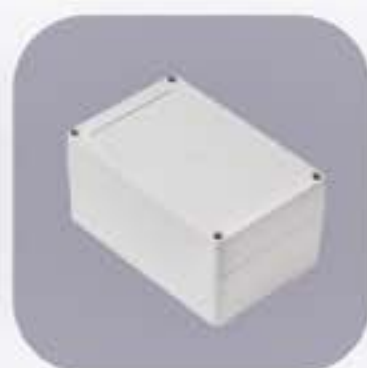
ZP150.100.75 MATERIAL: ABS/PC WITH GASKET H / W / L (mm): 75 / 100 / 150 AVAILABLE COLOURS: ■ ■
